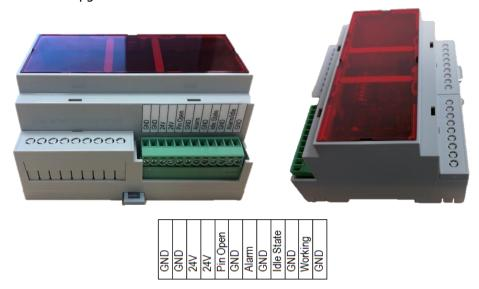
The Working signal can be directly connected and configured in KraussMaffei IMM machine as in the picture below.
