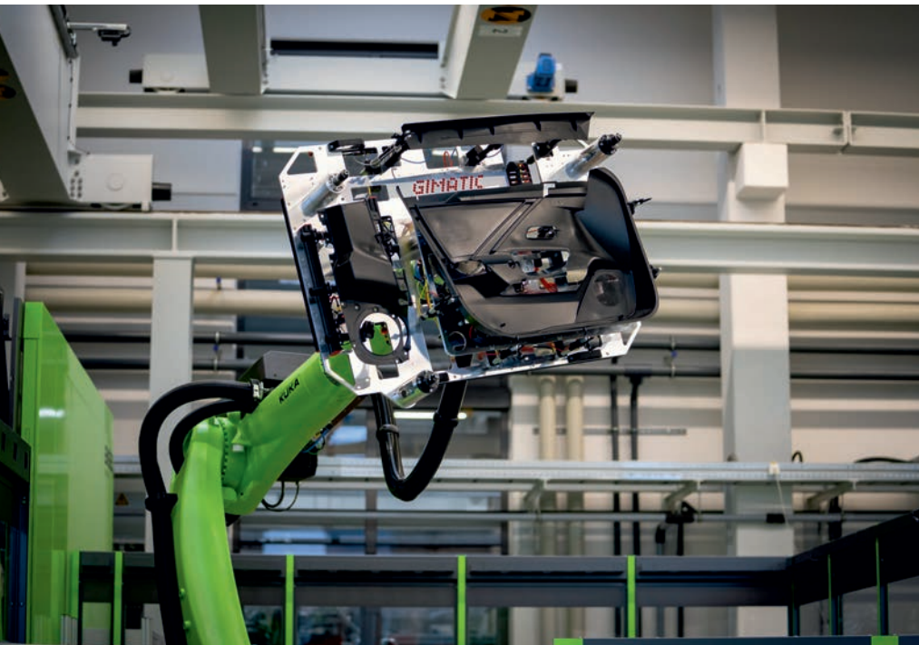
Three at once: a six-axis robot removes the final injection-molded assembly, consisting of door trim, map pocket and sill. © FoboHa / Christoph Raetzke
