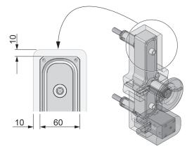
Installation of hardened insert opposite thrust pad is recommended. Not supplied with the hot runner system.
